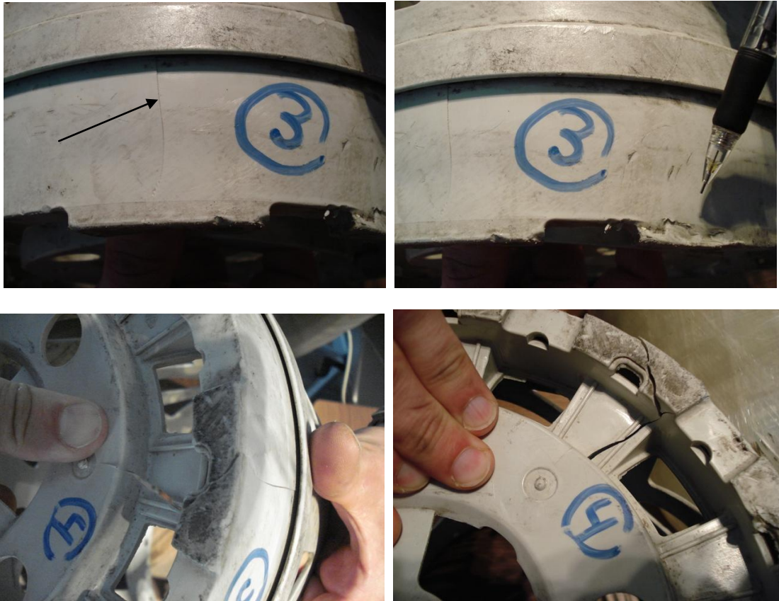
Figure 2b — Damage on casing base – not acceptable
