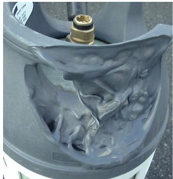
Figure 4 — Heat damage. This type of damage is not acceptable in any form
