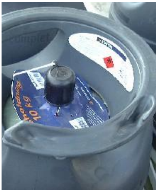
Figure 4 — Heat damage. This type of damage is not acceptable in any form
