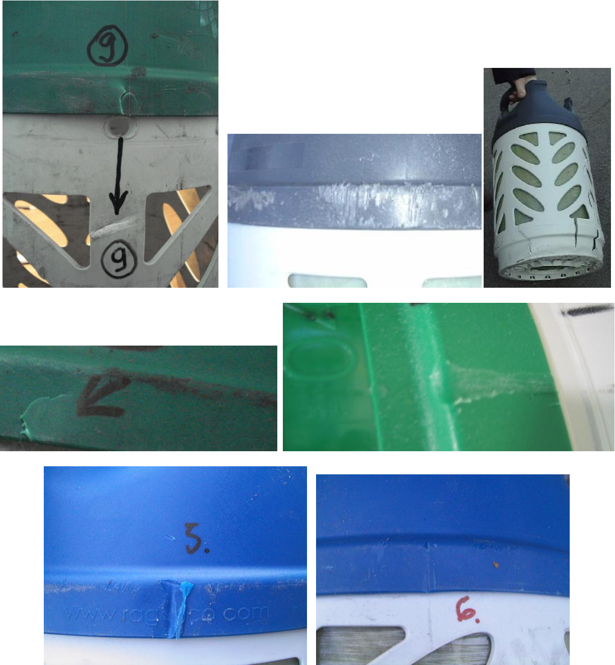
Figure 1a — Damage on casing “skirt”– not acceptable
