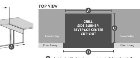
E Notch out width of countertop overhang should be cut back to the cabinet base to allow appliance to sit flush with base.
