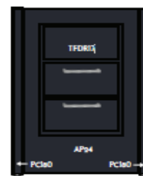
EXAMPLE OF A TFDR17 INSTALLED INTO A AP24 PANEL WITH PC180 CONNECTORS
