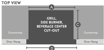
Notch out width of countertop overhang should be cut back to the cabinet base to allow appliance to sit flush with base.
