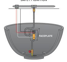
A thermocouple piloted system with safety valve that turns the gas off when there is a loss of flame. Easy ignition with manual spark igniter (included).
