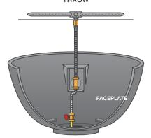
Easy lighting with a butane lighter or match. Variable flame height adjustment using a key valve.
