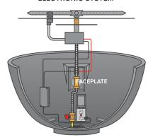
Our top of the line fully electronic ignition system. Ships with a GEO-30VDC power supply and an on/off toggle switch.
