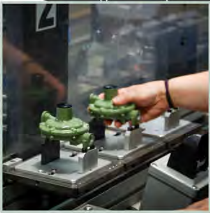
Plant 2 - Regulator Performance Testing
