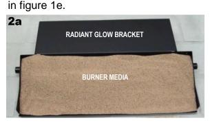
STEP 2: Fill the burner pan with the appropriate media as shown in figure 2a (sand for NG and vermiculite for LP) Install the grate over the burner pan. The front legs of the grate go around the burner pan and about 1" in front of the burner pipe as shown in figure 2b.
