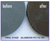
the finer particulate, water and heavy oils to strike their surfaces and each other, until they become large enough to be held in this media. Since most of the larger water, heavy oils and particulate molecules have been removed before entering this phase, this "micro" (5-micron) stage is able to work longer and more efficiently.
